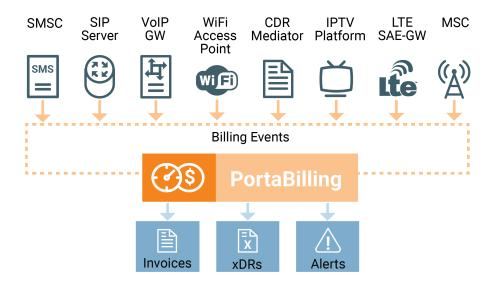
All this happens in real time, so that billing data is updated as soon as a session is completed (e.g. the customer hangs up his phone, or an SMS message is sent). PortaBilling® with Oracle Real Application Cluster provides a unified platform for multiple services, which allows you to use it to charge clients for their voice calls, text messages, and data transfers, thus effectively deploying triple-play on your network.
