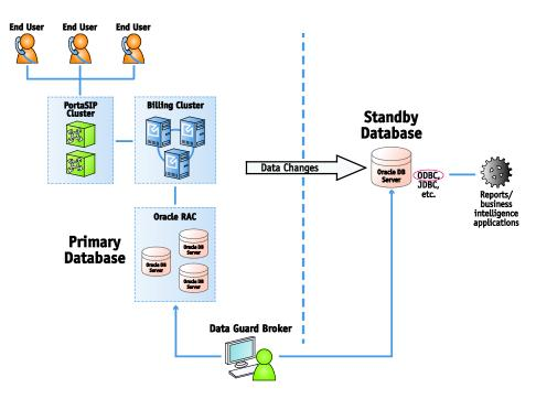
Furthermore, the same Data Guard node solution can be used when your standby database is located at a remote secondary site, miles away from your main data center.
