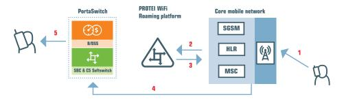
When someone dials the user's phone number (1), the mobile carrier addresses the PROTEI WiFi Roaming platform with a PRN (Provide Roaming Number) message (2). The PROTEI WiFi Roaming platform
