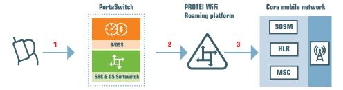
When a user connects to WiFi and the mobile application registers with PortaSwitch® (1), PortaSwitch® forwards the user's registration to the PROTEI WiFi Roaming platform (2). The PROTEI WiFi Roaming platform passes the user's current location to the user's mobile carrier within the LU (Location Update) message (3).
