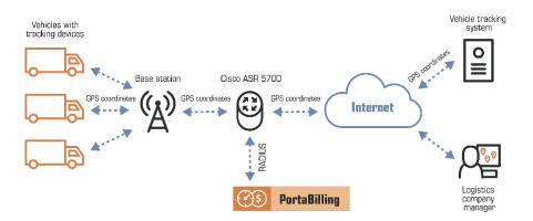
**NOTE**: Cisco ASR 5700 does not support PoD (Packet of Disconnect) and CoA (Change of Authorization) requests. To avoid overdrafts, use an external application to check the account's (device) balance / quota and disconnect an Internet session.
