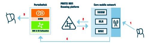
When someone dials the user's phone number (1), the mobile carrier addresses the PROTEI WiFi Roaming platform with a PRN (Provide Roaming Number) message (2). The PROTEI WiFi Roaming platform responds with the user's local roaming number and prefix (3) based upon which their mobile carrier routes the call to PortaSwitch® via SIP (4). PortaSwitch® then processes the call and delivers it to the user's mobile application (5).
