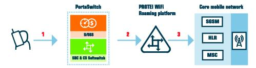
When a user connects to WiFi and the mobile application registers with PortaSwitch® (1), PortaSwitch® forwards the user's registration to the PROTEI WiFi Roaming platform (2). The PROTEI WiFi Roaming platform passes the user's current location to the user's mobile carrier within the LU (Location Update) message (3).
