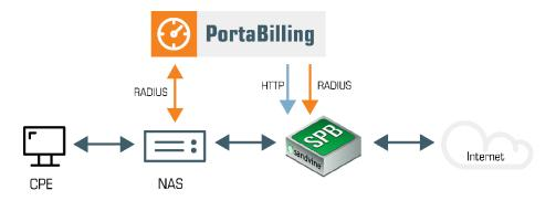
When an administrator creates a new customer in PortaBilling®, PortaBilling® sends the provisioning request to Sandvine SPB to create the new subscriber and assign a corresponding Internet access policy to it.
